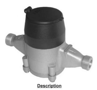
**Operation.** The C700 is an oscillating piston style, positive displacement water meter. The product utilizes a piston that water use rotates in a measuring chamber, each piston revolution being equivalent to a known volume of water. The piston movement is transferred by a magnetic drive to a straight reading sealed register which contains the appropriate reduction gearing.
